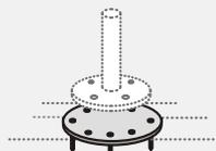
Base Plate 315mm $\phi$  - to bolt to timber decking
